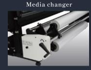
Three-roll media can be set. Anyone can easily, safely and efficiently switch between media simply by turning the handle.
