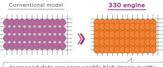
Increased dots per scan enable high image quality with fewer passes
